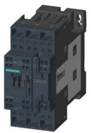
CONTACTOR, AC-3, 11KW/400V, 1NO+1NC, DC 48V, 3-POLE, SZ S0 SPRING-LOADED TERMINAL
