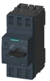
CIRCUIT-BREAKER SZ S00, FOR MOTOR PROTECTION, CLASS 10, A-RELEASE 5.5...8A, N-RELEASE 104A, SPRING-L. CONNECTION, STANDARD SW. CAPACITY
