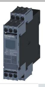
DIGITAL MONITORING RELAY SPEED MONITORING, FOR IO-LINK FROM 0.1 TO 2200 RPM OVERSHOOT AND UNDERSHOOT ON DELAY TIME TRIPPING DELAY TIME HYSTERESIS 0.1 TO 99 RPM 1 CHANGE-OVER CONTACT, SCREW TERMINAL
