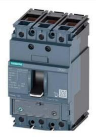
CIRCUIT BREAKER 3VA1 IEC FRAME 160 BREAKING CAPACITY CLASS S ICU=36KA @ 415 V 3-POLE, LINE PROTECTION TM240, ATAM, IN=125A OVERLOAD PROTECTION IR=87,5A ...125A SHORT CIRCUIT PROTECTION II=5...10 X IN CABLE CONNECTION
