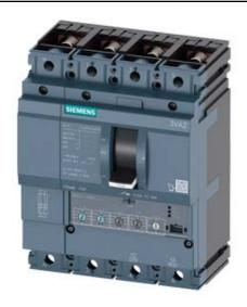
CIRCUIT BREAKER 3VA2 IEC FRAME 100 BREAKING CAPACITY CLASS M ICU=55KA @ 415 V 4POLE, LINE PROTECTION ETU330, LIG, IN=40A OVERLOAD PROTECTION IR=16A ...40A SHORT CIRCUIT PROTECTION II=1,5...12 X IN NEUTRAL PROTECTION ADJUSTABLE(OFF,100%) GROUNDFAULTPROTECTION IG=0,2... 1 X IN, TG=0,1/0,3MS BUSBAR CONNECTION
