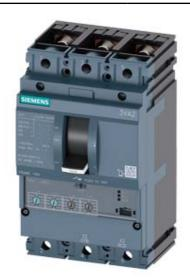
CIRCUIT BREAKER 3VA2 IEC FRAME 160 BREAKING CAPACITY CLASS H ICU=85KA @ 415 V 3POLE, LINE PROTECTION ETU330, LIG, IN=25A OVERLOAD PROTECTION IR=10A ...25A SHORT CIRCUIT PROTECTION II=1,5...12 X IN GROUNDFAULTPROTECTION IG=0,2... 1 X IN, TG=0,1/0,3MS BUSBAR CONNECTION
