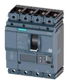
CIRCUIT BREAKER 3VA2 IEC FRAME 250 BREAKING CAPACITY CLASS C ICU=110KA @ 415 V 4POLE, LINE PROTECTION ETU850, LSI, IN=250A OVERLOAD PROTECTION IR=100A ...250A SHORT CIRCUIT PROTECTION ISD=0,6..10X IN, II=1,5..10X IN NEUTRAL PROTECTION ADJUSTABLE (OFF, UPTO 100%) BUSBAR CONNECTION
