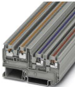
Sensor/actuator terminal block, with green light indicator, Connection method: Push-in connection, Cross section: 0.14 mm 2 - 1.5 mm 2 , AWG: 26 - 14, Width: 3.5 mm, Color: gray, Mounting type: NS 35/7,5, NS 35/15
