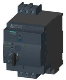
SIRIUS, COMPACT STARTER, REVERSING STARTER 690 V, 24 V AC/DC, 50 ... 60 HZ, 0.1 ... 0.4 A, IP20, MAIN CIRCUIT CONNECTION: SCREW TERMINAL, AUXILIARY CIRCUIT CONNECTION: PLUG-IN, W/O TERMINALS
