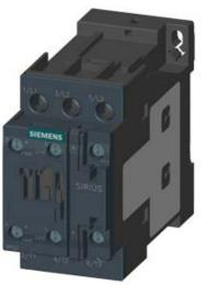
CONTACTOR, AC-3, 5.5KW/400V, 1NO+1NC, DC 110V, 3-POLE, SZ S0 SCREW TERMINAL
