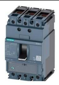
CIRCUIT BREAKER 3VA1 IEC FRAME 160 BREAKING CAPACITY CLASS H ICU=70KA @ 415 V 3-POLE, LINE PROTECTION TM220, ATFM, IN=160A OVERLOAD PROTECTION IR=112A ...160A SHORT CIRCUIT PROTECTION II=10 X IN CABLE CONNECTION
