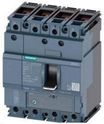
CIRCUIT BREAKER 3VA1 IEC FRAME 160 BREAKING CAPACITY CLASS M ICU=55KA @ 415 V 4-POLE, LINE PROTECTION TM220, ATFM, IN=20A OVERLOAD PROTECTION IR=14A ...20A SHORT CIRCUIT PROTECTION II=10 X IN NEUTRAL UNPROTECTED BUSBAR CONNECTION
