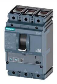
CIRCUIT BREAKER 3VA2 IEC FRAME 100 BREAKING CAPACITY CLASS C ICU=110KA @ 415 V 3POLE, LINE PROTECTION ETU320, LI, IN=40A OVERLOAD PROTECTION IR=16A ...40A SHORT CIRCUIT PROTECTION II=12 X IN CABLE CONNECTION
