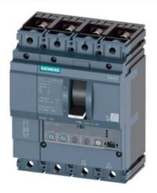
CIRCUIT BREAKER 3VA2 IEC FRAME 160 BREAKING CAPACITY CLASS M ICU=55KA @ 415 V 4POLE, LINE PROTECTION ETU330, LIG, IN=100A OVERLOAD PROTECTION IR=40A ...100A SHORT CIRCUIT PROTECTION II=1,5...12 X IN NEUTRAL PROTECTION ADJUSTABLE(OFF,50%,100%) GROUNDFAULTPROTECTION IG=0,2... 1 X IN, TG=0,1/0,3MS BUSBAR CONNECTION
