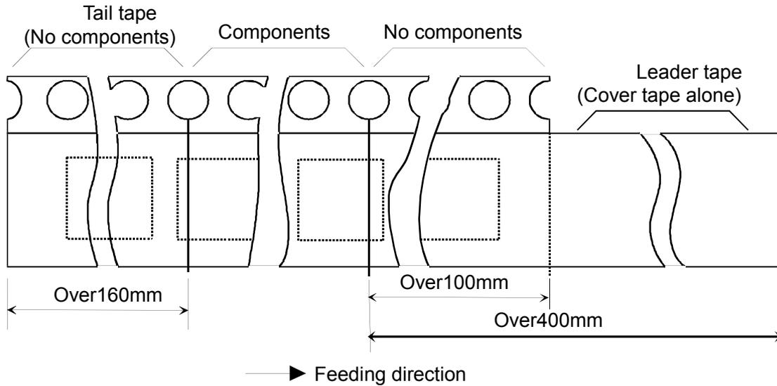
11-6. The tape for chips are wound clockwise, the feeding holes to the right side as the tape is pulled toward the user.
