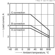
1-(2) Load current vs. ambient temperature characteristics
