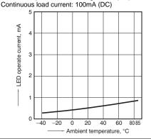
LED turn off current vs. ambient temperature characteristics
