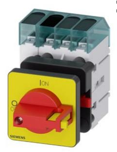
Switch disconnector 3LD3, main switch 3-polig + N, lu 16A operational switch at AC-23 A at 400 V 7,5 kW front mounted Base mounting with center-hole 22,5 mm knob-operated mechanism red/yellow 48 x 48 mm
