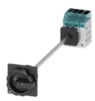
Switch disconnector 3LD3, main switch 3-polig + N, lu 25A operational switch at AC-23 A at 400 V 9,0 kW floor mounting Base mounting with door coupling center-hole 22,5 mm rotary operationg mechanism black  $66 \times 66 \text{ mm}$
