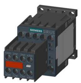
CONTACTOR, AC-3, 7.5KW/400V, 2NO+2NC, DC 24V, W. INTEGRATED DIODE 3-POLE, SZ S00 SCREW TERMINAL PERMANENT AUX. SWITCH
