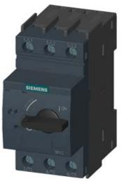
CIRCUIT-BREAKER SZ S0, FOR STARTER COMBINATION, RATED CURRENT 20A, N-RELEASE 260A, SCREW CONNECTION, STANDARD SW. CAPACITY
