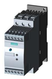
SIRIUS SOFT STARTER, SIZE S0, 38A, 18.5KW/400V, 40 DEGREES, 200-480V AC, 110-230V AC/DC, SCREW TERMINALS
