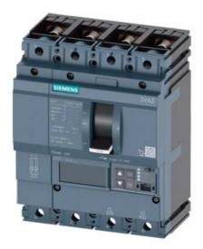
CIRCUIT BREAKER 3VA2 IEC FRAME 160 BREAKING CAPACITY CLASS H ICU=85KA @ 415 V 4POLE, LINE PROTECTION ETU850, LSI, IN=160A OVERLOAD PROTECTION IR=64A ...160A SHORT CIRCUIT PROTECTION ISD=0,6..10X IN, II=1,5..10X IN NEUTRAL PROTECTION ADJUSTABLE (OFF, UPTO 100%) BUSBAR CONNECTION
