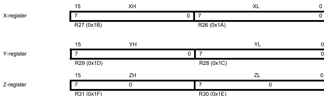
Figure 4-3. The X-, Y-, and Z-registers
