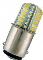
80100038771 LED Ba15d T15X36 24V AC/DC 1.8W (15W) 140lm 841
