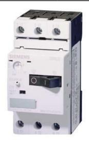
LEISTUNGSSCHALTER BGR. S00, FUER DEN MOTORSCHUTZ, CLASS 10, A-AUSL.0,28...0,4A,N-AUSL.5,2A, SCHRAUBANSCHLUSS, STANDARDSCHALTVERMOEGEN
