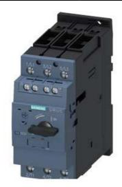
CIRCUIT BREAKER, SIZE S2, FOR MOTOR PROTECTION, CLASS 10, A-RELEASE 32...40A, N-RELEASE 585A, SCREW TERMINAL, STANDARD BREAKING CAPACITY W. TRANSV. AUX. SWITCH 1NO+1NC
