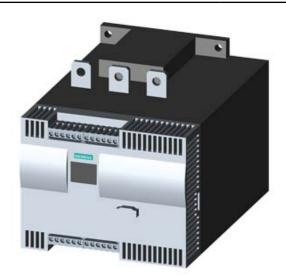
SIRIUS SOFT STARTER, VALUES WITH 460 V, 50 DEG., STANDARD: 215A, 150HP, INSIDE-DELTA CIRCUIT 3: 372A, 300HP, 200-460 V AC, 115 V AC, SCREW TERMINALS
