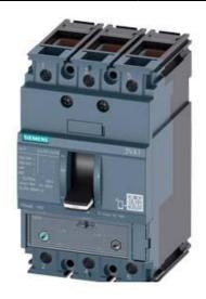
CIRCUIT BREAKER 3VA1 IEC FRAME 160 BREAKING CAPACITY CLASS N ICU=25KA @ 415 V 3-POLE, LINE PROTECTION TM240, ATAM, IN=20A OVERLOAD PROTECTION IR=14A ...20A SHORT CIRCUIT PROTECTION II=5...10 X IN CABLE CONNECTION
