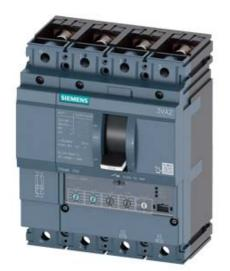
CIRCUIT BREAKER 3VA2 IEC FRAME 250 BREAKING CAPACITY CLASS L ICU=150KA @ 415 V 4POLE, LINE PROTECTION ETU330, LIG, IN=250A OVERLOAD PROTECTION IR=100A ...250A SHORT CIRCUIT PROTECTION II=1,5...10 X IN NEUTRAL PROTECTION ADJUSTABLE(OFF,50%,100%) GROUNDFAULTPROTECTION IG=0,2... 1 X IN, TG=0,1/0,3MS BUSBAR CONNECTION
