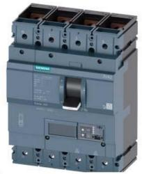
CIRCUIT BREAKER 3VA2 IEC FRAME 630 BREAKING CAPACITY CLASS M ICU=55KA @ 415 V 4-POLE, LINE PROTECTION ETU560, LSIG, IN=400A OVERLOAD PROTECTION IR=160A ...400A SHORT CIRCUIT PROTECTION ISD=0,6..10X IN, II=1,5..15X IN NEUTRAL PROTECTION ADJUSTABLE (OFF, UPTO 160%) GROUND-FAULT, SWITCHABLE IG=0,2... 1 X IN, TG=0,05-0,8MS BUSBAR CONNECTION
