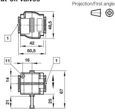
1 Main ports 1/4" or 3/8" ISO G/PTF 11 Exhaust port M5 at 3/2 valve only
