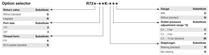
\*2) Outlet pressure can be adjusted to pressures in excess of, and less than, those specified. Do not use these units to control pressures outside of the specified ranges.
