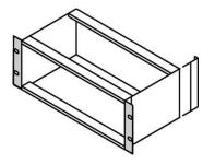
• 19" bracket is bolted laterally with the side panel to the horizontal rail
