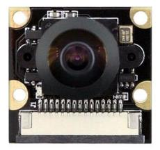
Raspberry Pi Wide Angle Camera Module is a low-cost Fisheye Lens, wider Field View, Camera module, designed for Raspberry Pi.
