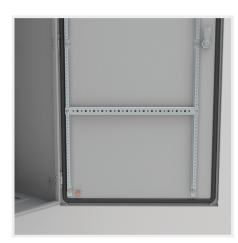
**Omschrijving:** Horizontal profiles with 25 mm hole pattern of 4.5 mm and 6.5 mm of diameter for the attachment and installation of equipment. They fit directly onto the MMDP door mounting profiles. They can also be mounted vertically onto two horizontal profiles. For doors with espagnolette locking system, profiles must be cut where indicated.
