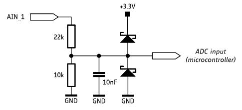
Figure 3.6 General purpose inputs (simplified input circuit)
