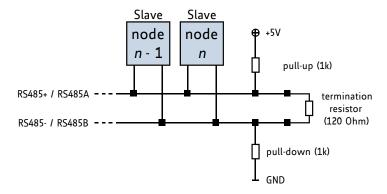
Figure 3.4 Bus lines with resistor network
