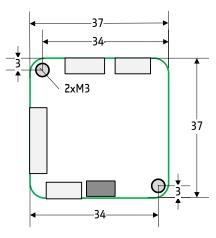
Figure 3.1 Dimensions of TMCM-1141 and position of mounting holes
