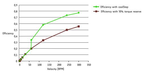
Figure 1.2 Energy efficiency example with coolStep
