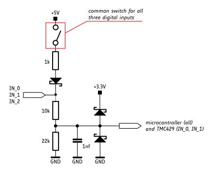
Figure 3.5 General purpose inputs (simplified input circuit)
