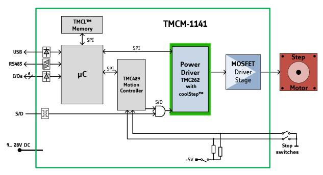
Figure 7.1 Main parts of the TMCM-1141
