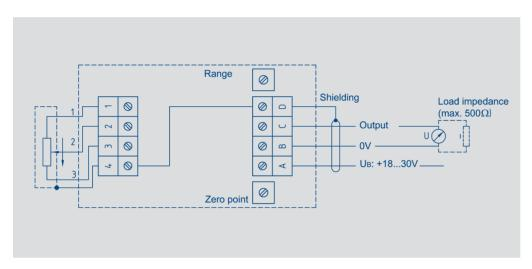
The output signal rises when the wiper is moved from position 1 to 3 (see connection diagram in the corresponding data sheet). For the reverse function, simply switch the connections 1 and 3 in the MUK housing.
