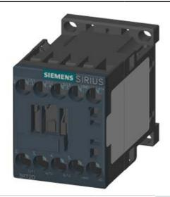
COUPLING RELAY, AC-3, 5.5KW/ 400V , 1NO, DC 24V, 0.7...1.25\*US, W. INTEGRATED DIODE 3-POLE SZ S00, SCREW TERMINAL
