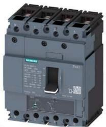
CIRCUIT BREAKER 3VA1 IEC FRAME 160 BREAKING CAPACITY CLASS N ICU=25KA @ 415 V 4-POLE, LINE PROTECTION TM220, ATFM, IN=40A OVERLOAD PROTECTION IR=28A ...40A SHORT CIRCUIT PROTECTION II=10 X IN NEUTRAL PROTECTION 100% BUSBAR CONNECTION
