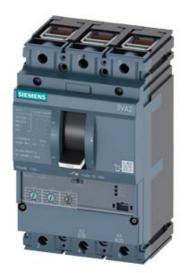
CIRCUIT BREAKER 3VA2 IEC FRAME 100 BREAKING CAPACITY CLASS M ICU=55KA @ 415 V 3POLE, LINE PROTECTION ETU320, LI, IN=25A OVERLOAD PROTECTION IR=10A ...25A SHORT CIRCUIT PROTECTION II=12 X IN CABLE CONNECTION
