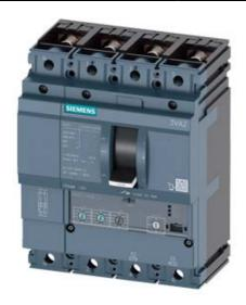
CIRCUIT BREAKER 3VA2 IEC FRAME 100 BREAKING CAPACITY CLASS M ICU=55KA @ 415 V 4POLE, LINE PROTECTION ETU320, LI, IN=63A OVERLOAD PROTECTION IR=25A ...63A SHORT CIRCUIT PROTECTION II=12 X IN NEUTRAL PROTECTION ADJUSTABLE(OFF,100%) BUSBAR CONNECTION
