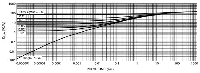
Figure 13. Transient Thermal Impedance
