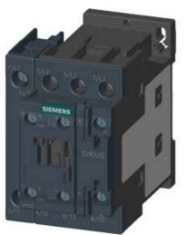
4NO CONTACTOR, AC1: 50A AC 230V 50/60HZ 4-POLE, 4NO, SZ: S0, SCREW TERMINAL 1NO+1NC INTEGR.
