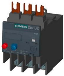
OVERLOAD RELAY 11...16 A FOR MOTOR PROTECTION SZ S0, CLASS 10, F. MOUNTING ONTO CONTACTOR MAIN CIRCUIT: RING CABLE LUG AUX. CIRCUIT: RING CABLE LUG MANUAL-AUTOMATIC-RESET
