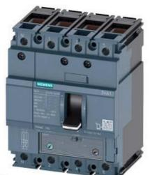
CIRCUIT BREAKER 3VA1 IEC FRAME 160 BREAKING CAPACITY CLASS M ICU=55KA @ 415 V 4-POLE, LINE PROTECTION TM240, ATAM, IN=20A OVERLOAD PROTECTION IR=14A ...20A SHORT CIRCUIT PROTECTION II=5...10 X IN NEUTRAL UNPROTECTED CABLE CONNECTION
