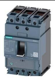
CIRCUIT BREAKER 3VA1 IEC FRAME 160 BREAKING CAPACITY CLASS N ICU=25KA @ 415 V 3-POLE, LINE PROTECTION TM220, ATFM, IN=40A OVERLOAD PROTECTION IR=28A ...40A SHORT CIRCUIT PROTECTION II=10 X IN CABLE CONNECTION
