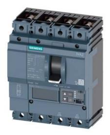
CIRCUIT BREAKER 3VA2 IEC FRAME 250 BREAKING CAPACITY CLASS L ICU=150KA @ 415 V 4POLE, LINE PROTECTION ETU550, LSI, IN=250A OVERLOAD PROTECTION IR=100A ...250A SHORT CIRCUIT PROTECTION ISD=0,6..10X IN, II=1,5..10X IN NEUTRAL PROTECTION ADJUSTABLE (OFF, UPTO 100%) BUSBAR CONNECTION
