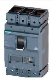
CIRCUIT BREAKER 3VA2 IEC FRAME 400 BREAKING CAPACITY CLASS M ICU=55KA @ 415 V 3-POLE, LINE PROTECTION ETU550, LSI, IN=250A OVERLOAD PROTECTION IR=100A ...250A SHORT CIRCUIT PROTECTION ISD=0,6..10X IN, II=1,5..12X IN NEUTRAL PROTECTION OPTIONAL WITH EXT. CT;UPTO 160% BUSBAR CONNECTION
