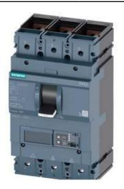
CIRCUIT BREAKER 3VA2 IEC FRAME 630 BREAKING CAPACITY CLASS C ICU=110KA @ 415 V 3-POLE, LINE PROTECTION ETU550, LSI, IN=500A OVERLOAD PROTECTION IR=200A ...500A SHORT CIRCUIT PROTECTION ISD=0,6..10X IN, II=1,5..14X IN NEUTRAL PROTECTION OPTIONAL WITH EXT. CT;UPTO 160% BUSBAR CONNECTION
