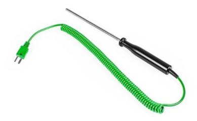
Rounded tip suitable for semi solid and liquid temperature measurement Mineral Insulated Immersion Probe with a rounded tip suitable for semi solid and liquid temperature measurement. Comprising of a handle, 2 metre coiled cable and Type mini plug. A semi flexible construction allows the probe to be bent or shaped for hard to reach applications. They are suitable for use in corrosive material tests and high temperature molten metal measurements.
