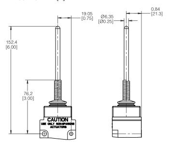
Figure 5. MICRO SWITCH™ BX SERIES CAT WHISKER WOBBLE, HEAD CODE K • mm [in]
