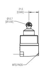
Figure 11. MICRO SWITCH™ BX SERIES ADJUSTABLE TOP PIN PLUNGER, HEAD CODE V • mm [in]
