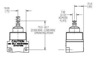
Figure 7. MICRO SWITCH™ BX SERIES TOP PIN PLUNGER, **HEAD CODE C** • mm [in]
