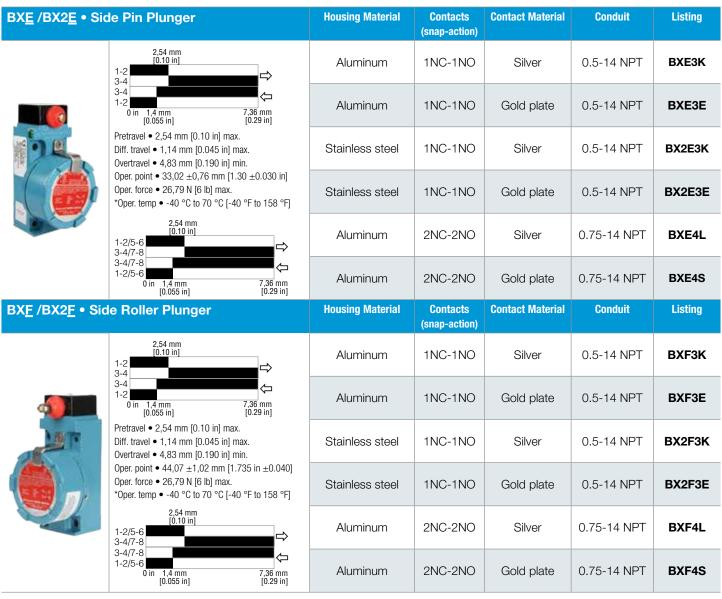
Contact closed ■; Contact open □ NOTE: Same polarity each pole.
