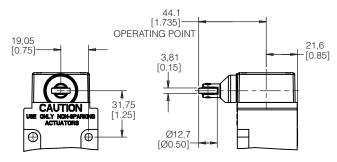
Figure 12. MICRO SWITCH™ BX SERIES ADJUSTABLE SIDE PIN PLUNGER, HEAD CODE W • mm [in]
