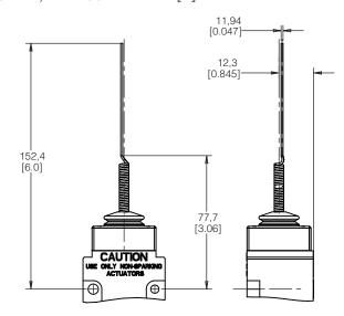
Figure 6. MICRO SWITCH™ BX SERIES TOP ROTARY, **HEAD CODE B** • mm [in]
