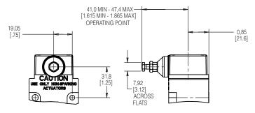
Figure 13. MICRO SWITCH™ BX2 Series Side Rotary Product Dimensions • mm [in] SIDE ROTARY - HEAD CODES: A, P, AND R
